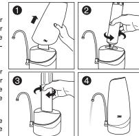
Note: During filter replacement, it's normal for residue water to flow out from insert at water filter base after the old cartridge is removed.
